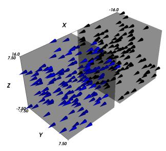
Time T=1e-10s=0.1ns: Cobalt is already pointing up, i.e. in the direction of the anisotropy axis, while Permalloy has just started to rotate.
