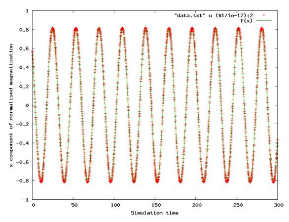
The values for B in the fit, which corresponds to the unknown period T, is initially set to 30 in order to help Gnuplot fit the curve. Such fit on T gives the value 28.4293; this value corresponds to 0.0284293 ns when rescaled by the 10e12 factor used for the plotting, and shows a difference starting from the 5th digit when compared to the analytical solution of 0.0284284 ns.
