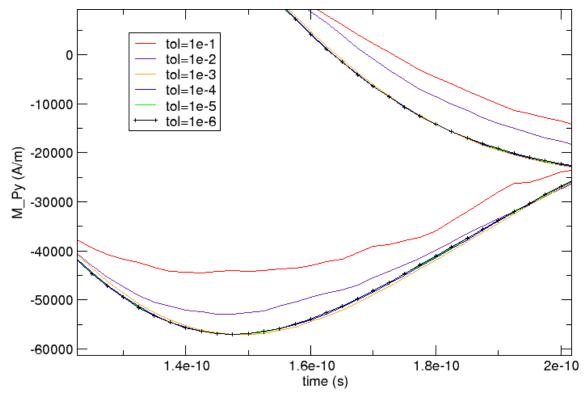
The better resolution reveals that there is a clear deviation of the various curves: the red (0.1), indigo (0.01) and yellow (1e-3) curves approach the black (1e-6) curve in this order. The blue (1e-4) and green (1e-5) curves appear to coincide with the black reference curve.
