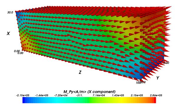
Because we have saved all fields (not just the magnetisation), we can also study other properties. For example, the following image shows the demagnetisation field as vectors (and the legend refers to the magnitude of the vectors), as well as the magnetic scalar potential (as a stack of isosurfaces). Because the demagnetisation field is the (negative) gradient of the scalar potential, the vectors are perpendicular on the isosurfaces:
