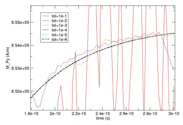
We conclude that we should use a tolerance of at most 1e-3 for this simulation; better 1e-4 or smaller.
