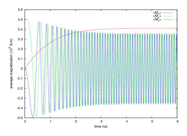
The sinusoidal dependence of the y and z magnetisation components suggests that the magnetisation rotates around the nanopillar axis with a frequency which increases to approach its maximum value.
