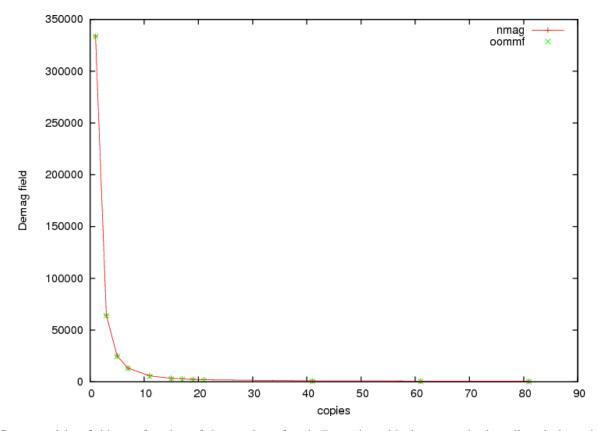
Demagnetising field as a function of the number of periodic copies with the magnetisation aligned along the periodic axis.
