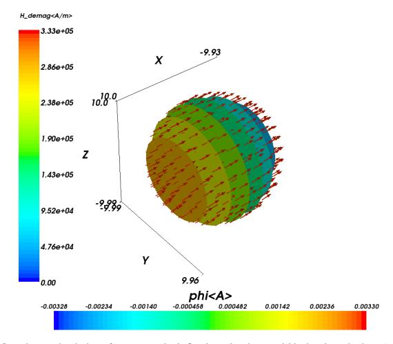
It can be seen that the isosurfaces are completely flat planes (i.e. the potential is changing only along x) and the demagnetisation field is perpendicular to the isosurfaces. The color bar on the left refers to the magnitude of the demagnetisation field which is expressed in Ampere per meter, as can be seen from the label <A/m>. (Note that all the H\_demag arrows are colored red as they have identical length.)
