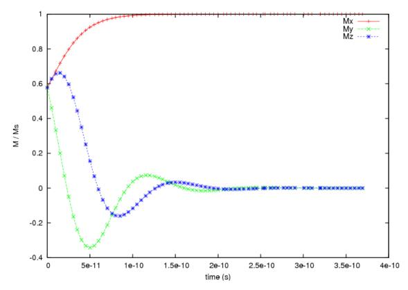
From this plot we can see that with using only the unit cell the magnetisation aligns along the x-axis at equilibrium.
