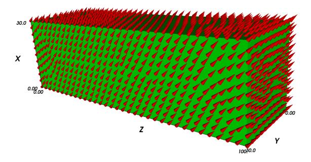
The "final" configuration shows that the magnetisation aligns along the z-direction. The coloured surface shows the x-component of the magnetisation (and the colorbar provides the scale). It can be seen that the magnetisation at position z=100 nm goes into a flower state to minimise the overall energy. (Note that, strictly speaking, this system is not yet in a meta-stable state after 300 ps – but already quite close.):
