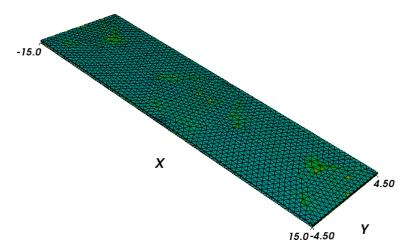
The mesh is contained in periodic.nmesh and has been produced using Netgen (from periodic.geo) and the *nmeshmirror* command to create required periodic structure
