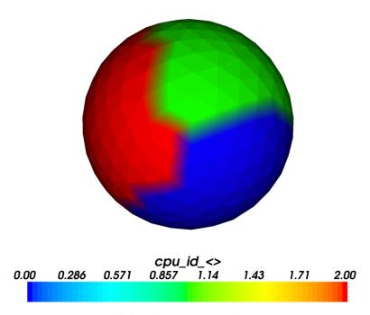
The figure shows that the sphere has been divided into three areas which carry values 0, 1 and 2 (corresponding to the MPI CPU rank which goes from 0 to 2 for 3 CPUs). Actually, in this plot we can only see the surface nodes (but the volume nodes have been partitioned accordingly).
