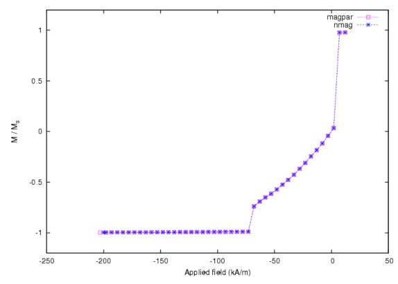
and we can see that the results from *nsim* match those from magpar. The magnetisation configurations during the switching process are shown in the following snapshots:
