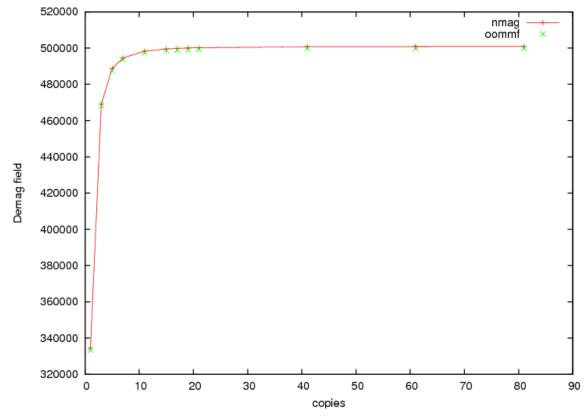
Demagnetising field as a function of the number of periodic copies with the magnetisation aligned along an axis orthogonal to the periodic one.
