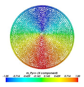
Figure 2.3: Magnetisation configuration for a decreasing applied field of 10 kA/m.
