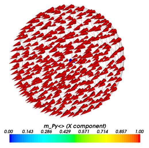
We can see one blue cone in the centre of the sphere - this is the one site that he have modified to point in the y-direction (whereas all other cones point in the x-direction).
