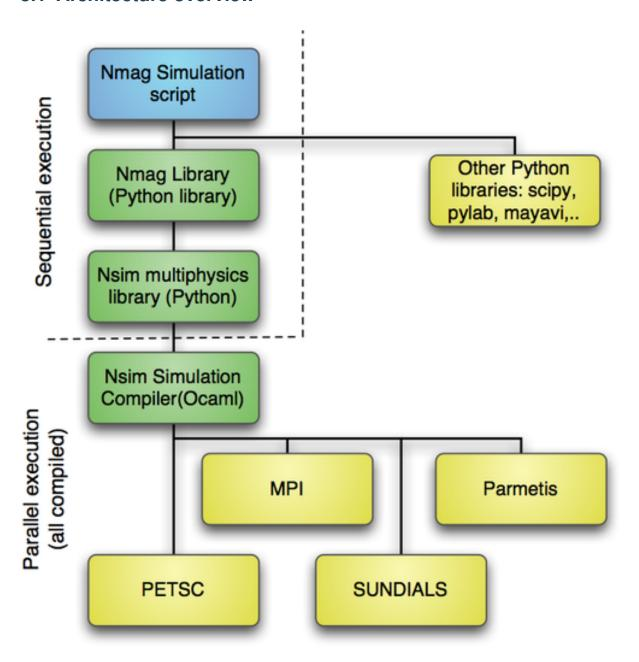
The Nmag environment that is described in this manual is shown as the blue box labelled Nmag Simulation Script. This is importing the nmag library – which is a Python library. This in turn, is built on the Nsim library Python module. The nsim Python module uses compiled code which is written in Objective Caml. At this level the execution can be parallel and this is also used to link together existing libraries (yellow boxes).
