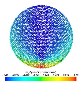
Figure 2.5: Magnetisation configuration for a decreasing applied field of -95 kA/m.
