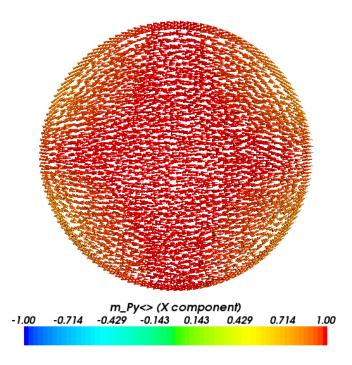
Figure 2.1: Magnetisation configuration for a decreasing applied field of 20 kA/m. The x-axis is increasing from left to right for this and the subsequent plots.
