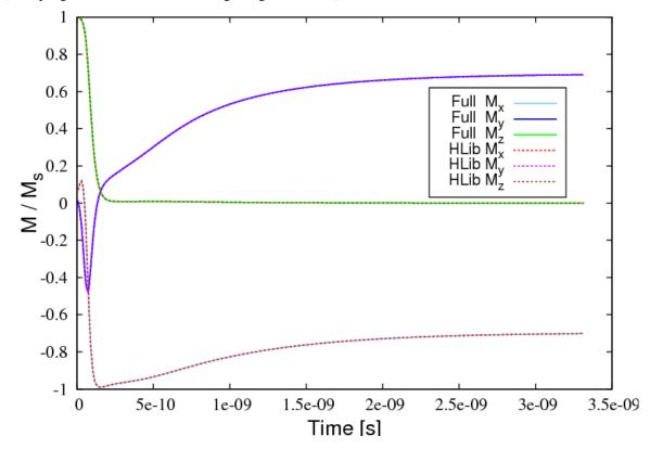
The magnetisation field moves from its out-of-plane configuration into the plane and relaxes into a high remanent state, which is aligned along the diagonal of the square base. The plot below shows a 3d visualisation of the relaxed magnetisation field (obtained with Mayavi2) for a thin film with an edge length of 130 nm.
