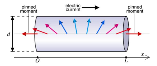
wall. We then study how such an "artificial" domain wall interacts with a current flowing throughout the cylinder, along its axis.
