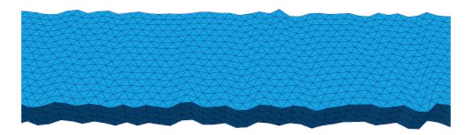
This figure shows a smooth nanowire (top), and then the same mesh after having been distorted using the nmesh command shown above. The figure is taken from  $^2$ .
