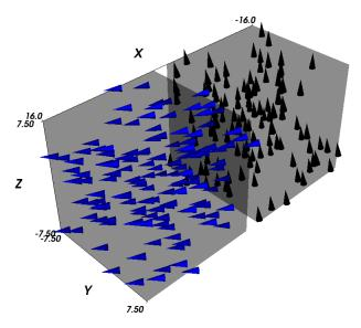
Time T=0.3ns: Cobalt has reached its final configuration (pointing up) and Permalloy is still rotating, but already pointing down (to minimise the interaction energy between the cubes to the demagnetisation stray fields).
