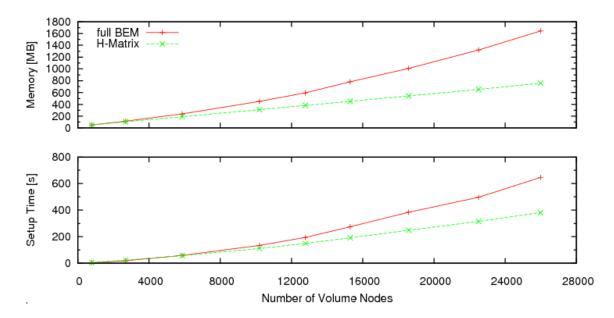
Besides the savings in memory, hierarchical matrices also reduce the time needed for the simulation setup considerably (see the bottom graph).
