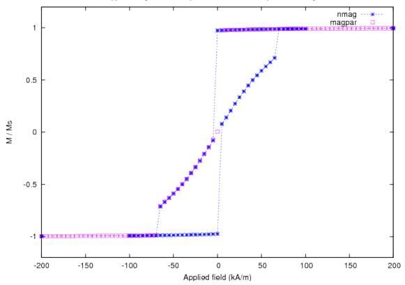
Here we can see a slight difference between nmag and Magpar in the location of the switching point, probably due to different tolerances in both programs when determining time integrator convergence.
