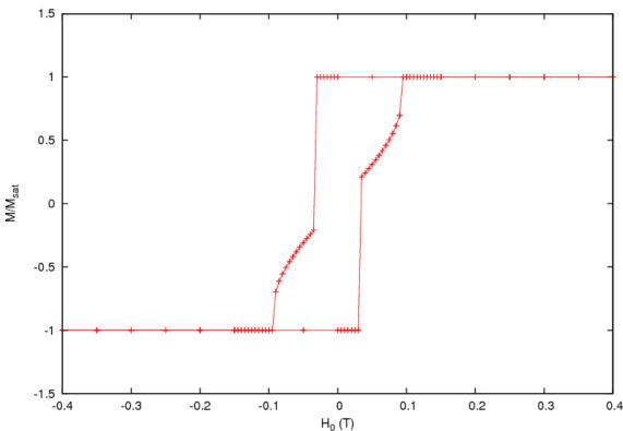
During the switching the system falls into an intermediate state, where the magnetisation is nearly aligned with the anisotropy easy axis.
