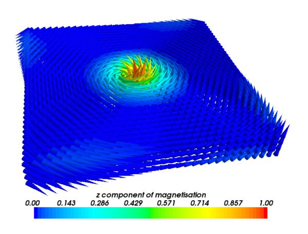
The relaxed vortex is much smaller than the initial one. The important thing to notice is that such a magnetisation configuration has now been saved into the file vortex\_m.h5 which will be used as the initial magnetisation for part II of this simulation, where we study the current driven dynamics of the vortex.
