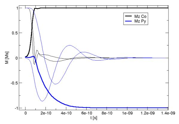
The blue lines represent the (soft) permalloy and the black lines show the (hard) cobalt. Each thick line denotes the z-component of the corresponding material.
