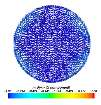
Figure 2.6: Magnetisation configuration for a decreasing applied field of -100 kA/m.
