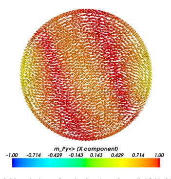
Figure 2.2: Magnetisation configuration for a decreasing applied field of 15 kA/m.
