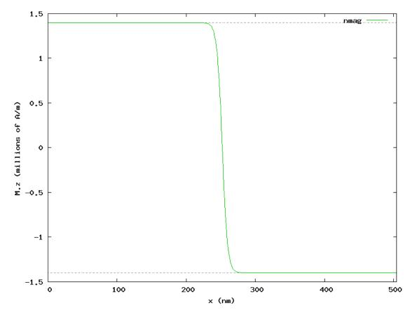
The figure shows also that the Bloch domain wall is well localized at the center of the bar, in the region where x goes from 200 to 300 nm.
