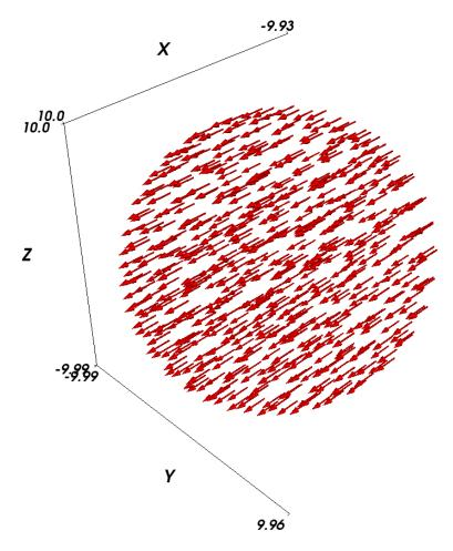
The magnetisation is pointing in positive x-direction because we initialised the magnetisation in this orientation by issuing the command  $sim.set_m([1,0,0])$ .
