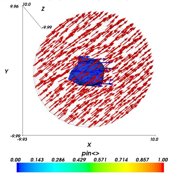
The blue blob in the center of the sphere is the collection of those tetrahedra that have corners just inside the 4nm sphere. Because we have not generated the mesh to have nodes coinciding with the 4nm sphere, the shape of the blue region is not particularly spherical.
