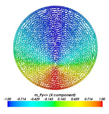
Figure 2.4: Magnetisation configuration for a decreasing applied field of -30 kA/m.
